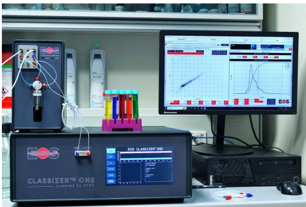
An example of set-up Single Particle Extinction and Scattering (SPES)
